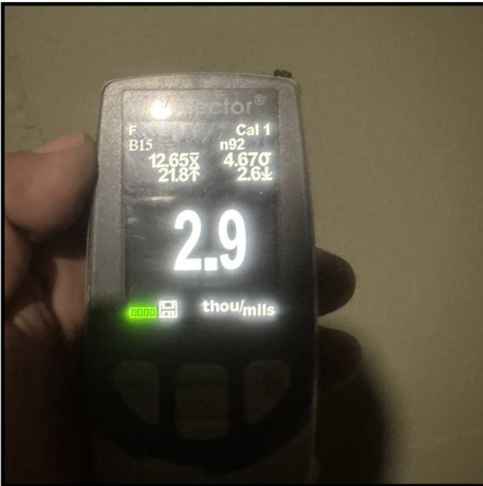
Dry film thickness of prime coat meets product standards
