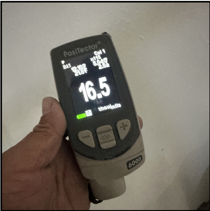
Dry film thickness of interior coatings meet manufacturer standards
