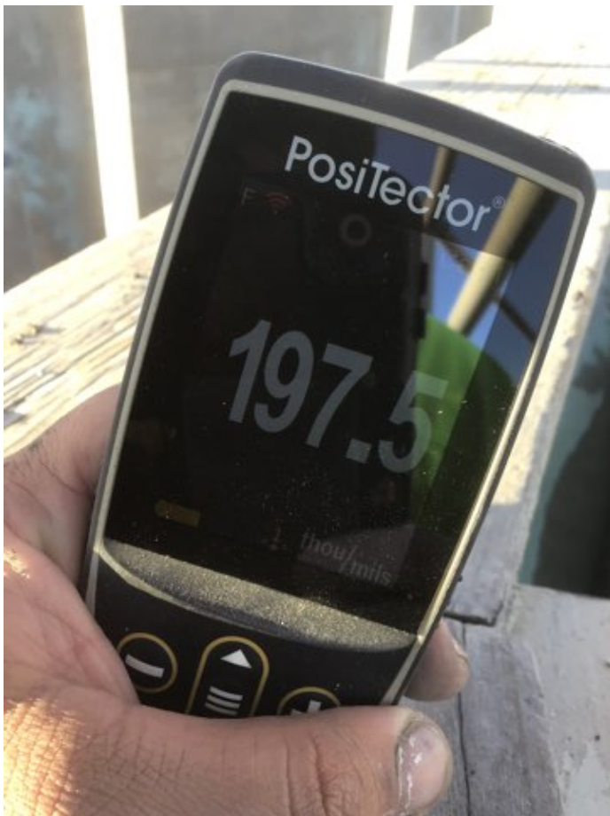
Photo Description: Mil reading of 197.5 before surface prep begins.
