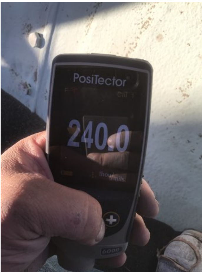
Photo Description: Mil reading of 240 before surface prep begins.
