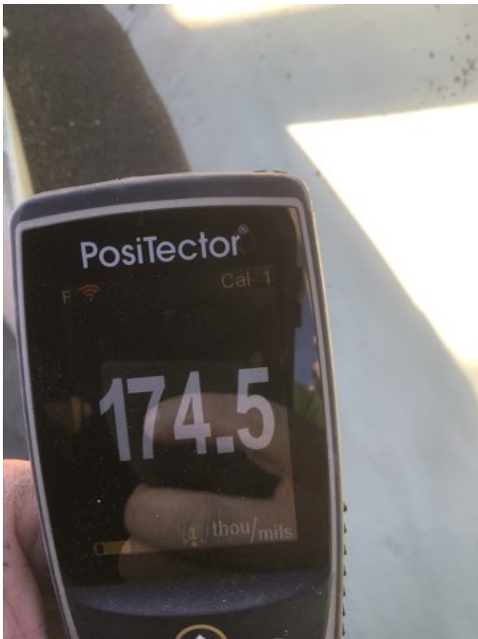
Photo Description: Mil reading of 174.5 before surface prep begins.
