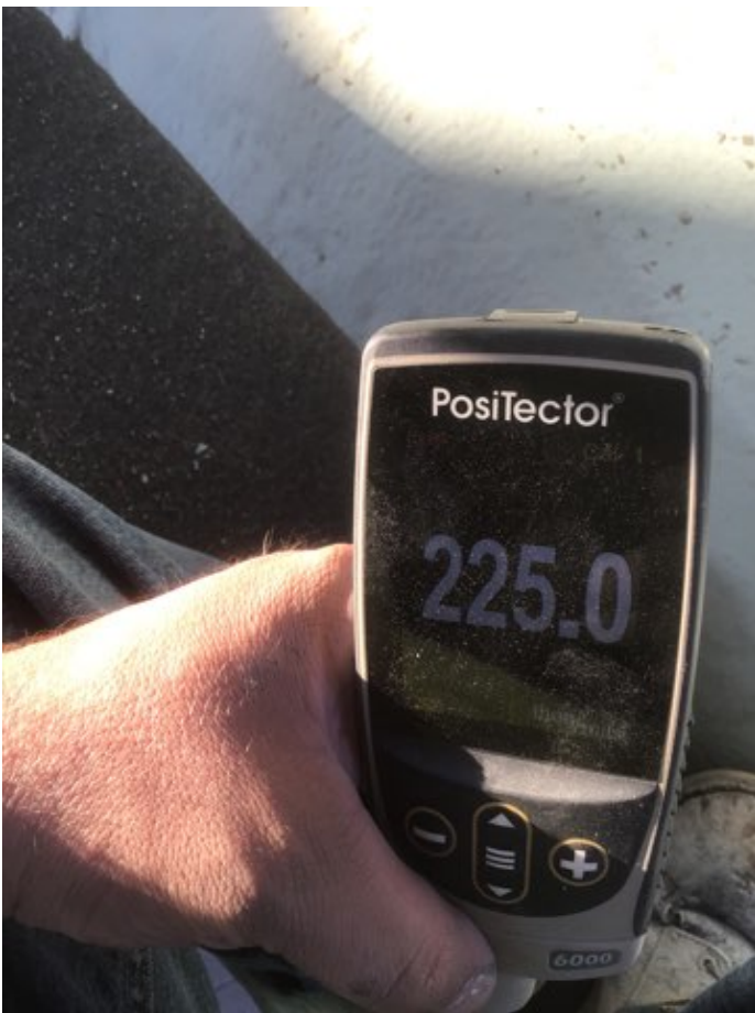
Photo Description: Mil reading of 225 before surface prep begins.
