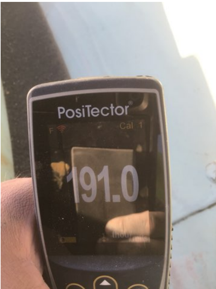
Photo Description: Mil reading of 191 before surface prep begins.
