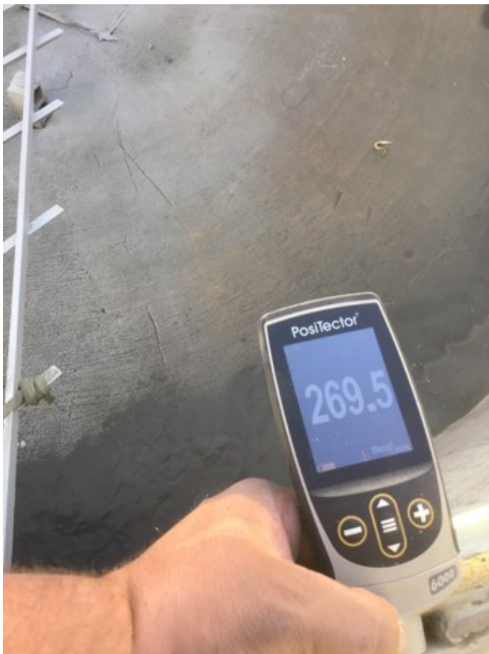
Photo Description: Mil reading of 269.5 before surface prep begins.
